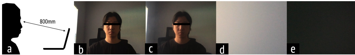
Fig. 2. This figure demonstrates webcam view difference between with and without PDLC-SWC. Macbook Pro Late 2016 models' FaceTime HD is used for testing: (a) the test distance between a user and a webcam is around 800mm with a sitting position; (b) webcam view without PDLC-SWC; (c) webcam view with PDLC-SWC when the PDLC film turns transparent in a bright environment; (d) webcam view with PDLC-SWC when the PDLC film turns opaque in a bright environment and (e) in a dark environment.
