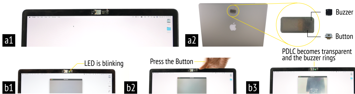
Fig. 5. This figure shows how HSWC works: (a1) HSWC is attached same as PDLC-SWC; (a2) The button and buzzer are contained in a container and are attached on the laptop lid; (b1) Even if a webcam is activated, the PDLC film stays opaque and the LED indicator is blinking, which indicates that the cover is closed; (b2,b3) A user needs to press the button manually to unblock the webcam.
